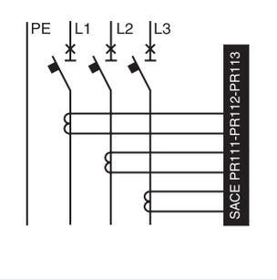
For users that do not use the neutral (e.g.: asynchronous motors) and, for systems with non-distributed neutral in general.
