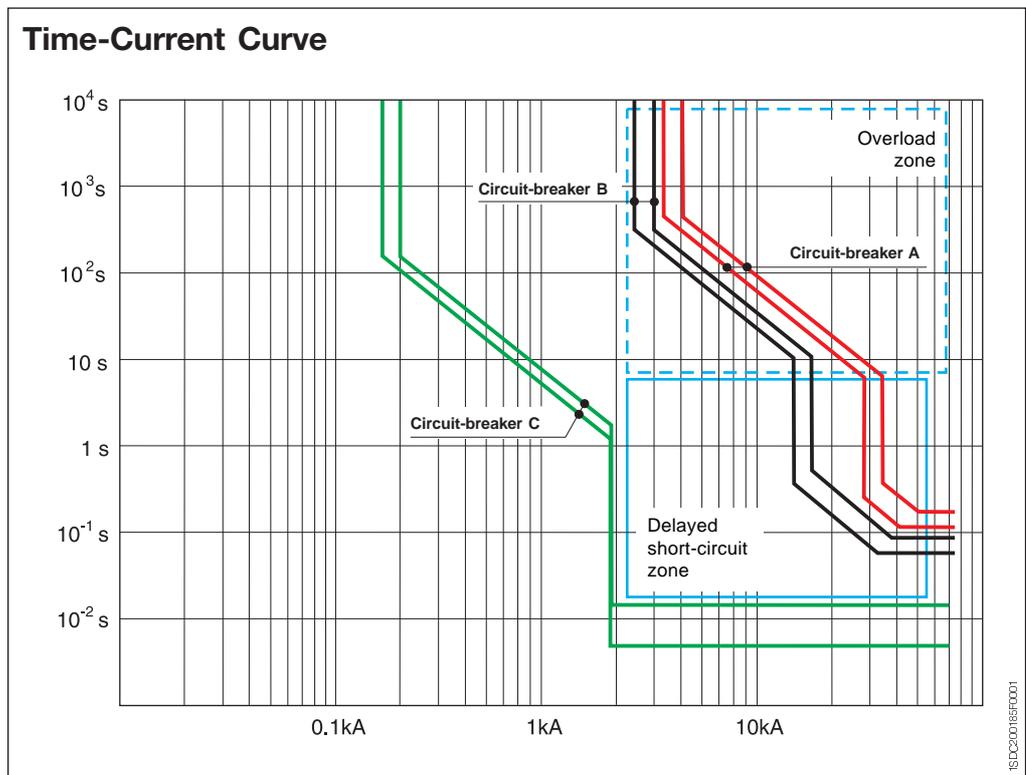
**Zone discrimination**, applicable to protection functions S, G and D. This type of discrimination allows shorter trip times for the circuit-breaker closest to the fault than in the case of time discrimination.
