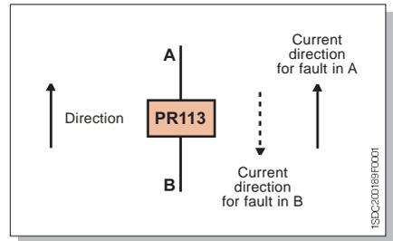
With reference to the figure below, for the circuit breaker QF1 if a fault occurs at point B the current will flow in direction A-B, discordant to the reference direction: the trip time will be Bw. Similarly, for a fault in A, the current direction will be B-A in agreement with the reference direction: the trip time will be Fw.
