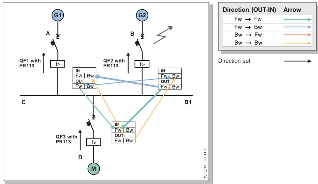
3) for a fault in C, the circuit-breakers QF1 and QF2 are traversed by a current with direction discordant to the setting, while QF3 is traversed by a current in the same direction as the setting. No circuit-breaker, however, is locked and thus all will trip according to the selected times. The figure below shows only the connections, as no lock signal is active.
