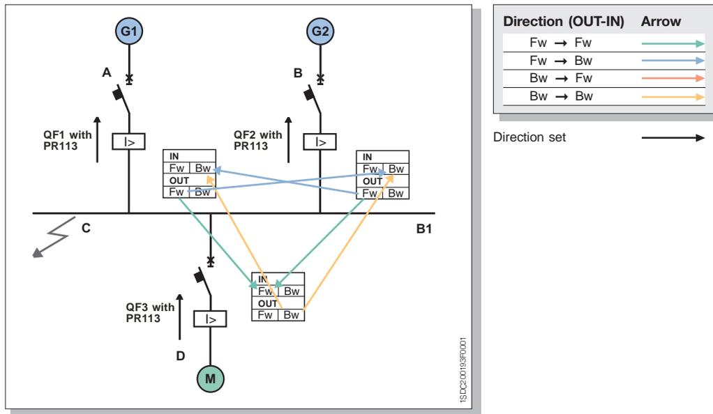
4) for a fault in D, the circuit-breaker QF3 is traversed by a current from the busbar B1; this current flows in a direction discordant to the setting. The OUT bus Bw of QF3 locks the IN Bus Bw of the circuit-breakers QF1 and QF2: both are traversed by fault currents discordant to the direction set. The figure below shows the connections between the relays, and the thicker arrows indicate the active lock signals in addition to the connections.
