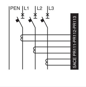
For TN-C systems (the neutral cannot be interrupted because it also acts as the protection conductor).
