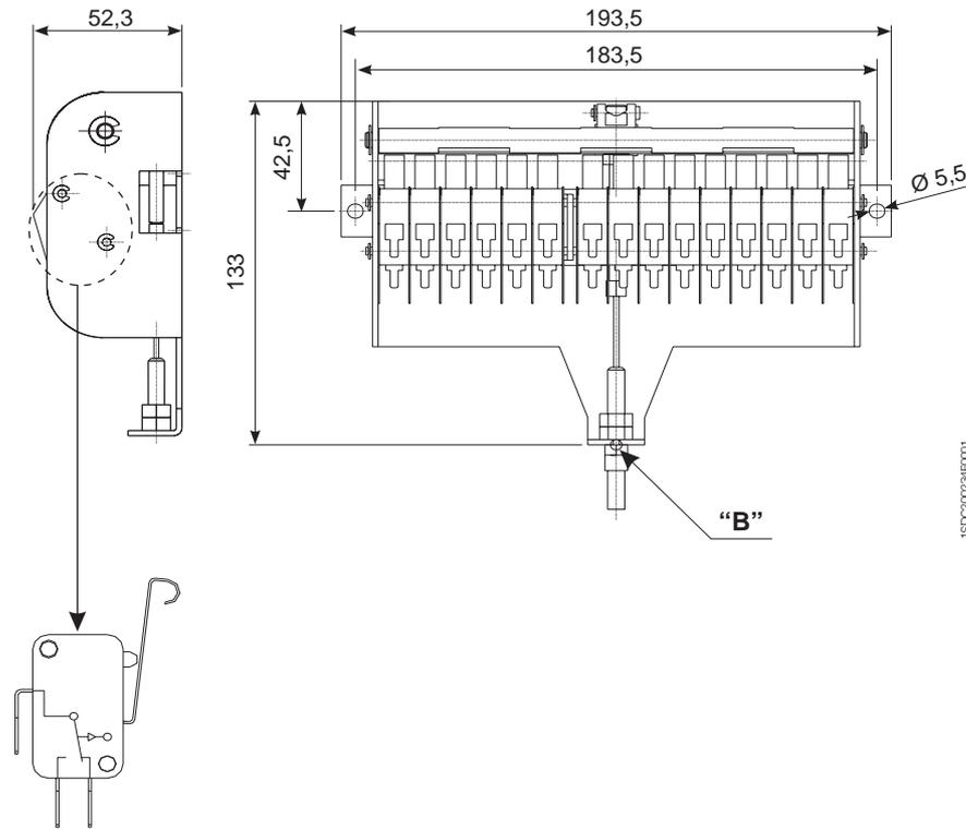
A flexible cable 650 mm long is available from point "A" to point "B".
