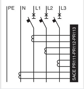
Current transformers can be installed on the external neutral of five-wire systems (TN-S) with 3-pole circuit-breakers.
