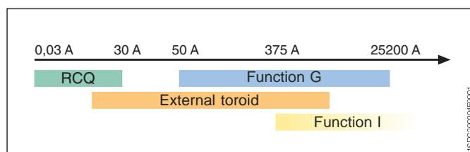
The figure shows which function of the electronic release or device to use based on the fault current.
