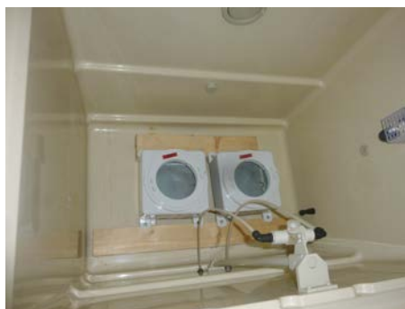
Fig. 20 Enclosures tested in salt mist
