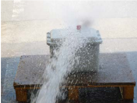
Fig. 21 IP X6 protection degree test
